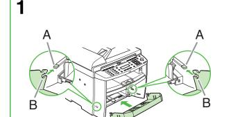
Align the guides (B) on the both edges of the paper cassette to the protrusions (A) inside the machine.
